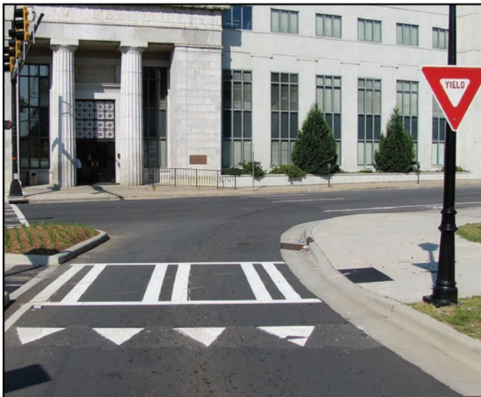
Advanced yield line (shark's teeth) denote yield point to motorists
