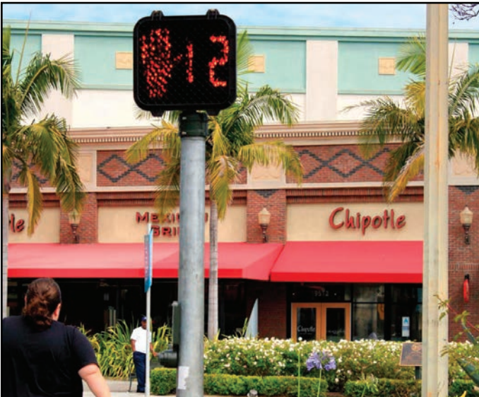
Pedestrian countdown signal shows there are 12 seconds left to cross before signal will turn
