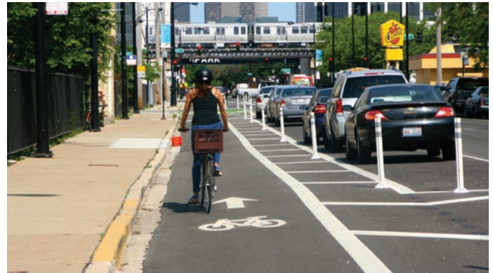
Parking-Protected Bike Lanes with Flexible Delineator Posts
