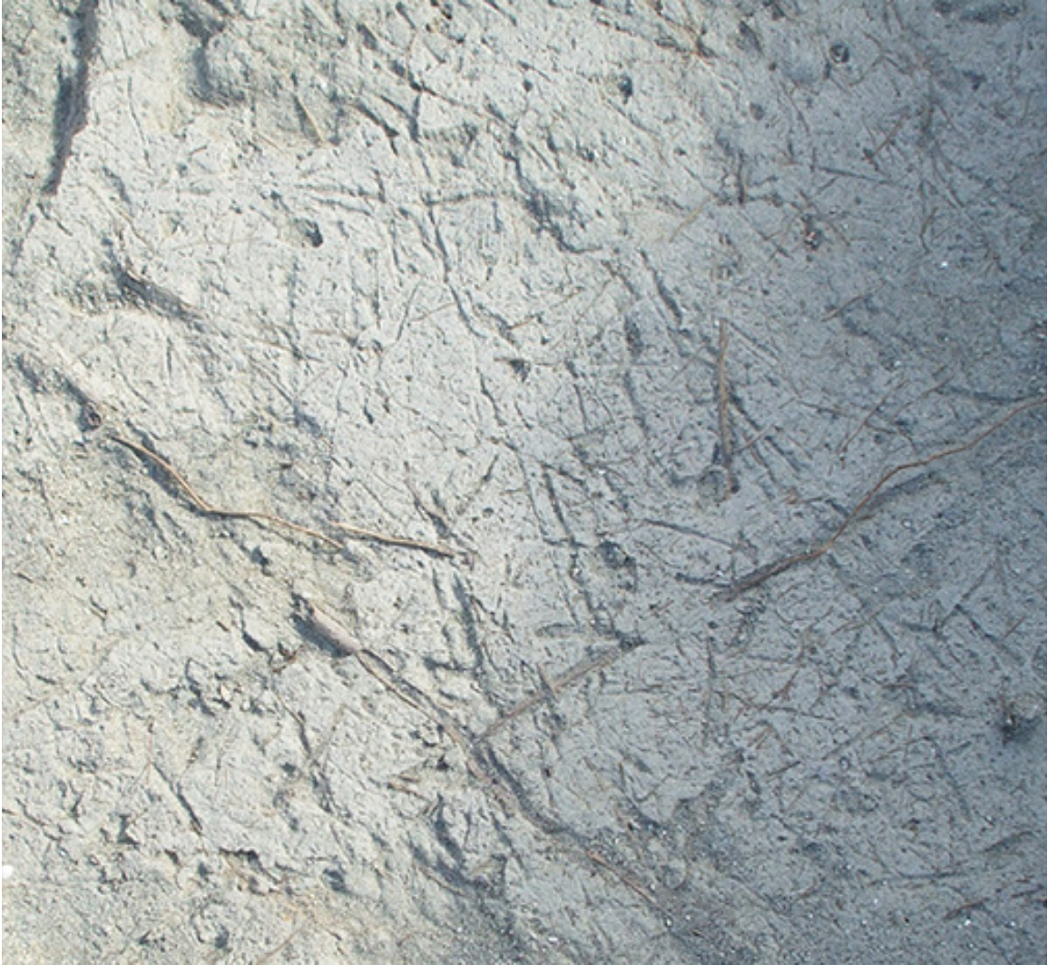
Photo 23: Level IV (somewhat compacted, very fine sandy silt with clay) with embedded plant roots seeking moisture (Unit 24A floor)
