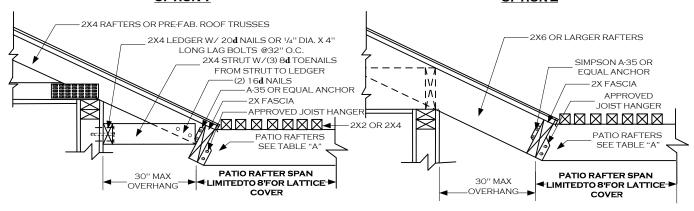
NOTE: VERIFY STRUCTURAL SOUNDNESS OF ROOF RAFTERS FOR DECAY OR TERMITE DAMAGE, AND REPLACE WITH LIKE MATERIALS AS NEEDED, AFTER CONSULTATION WITH THE BUILDING DEPARTMENT.
