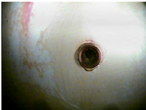
33. Sample Port Interior Corrosion
