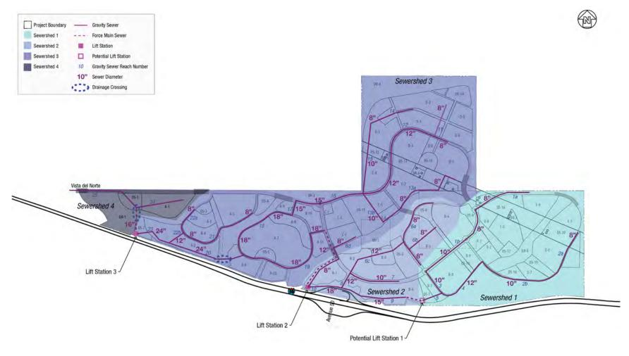
**FIGURE 2-16: CONCEPTUAL SEWER PLAN**
