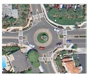
entry points and counterclockwise circulation around the center-island, these devices will limit speed and calm traffic.
