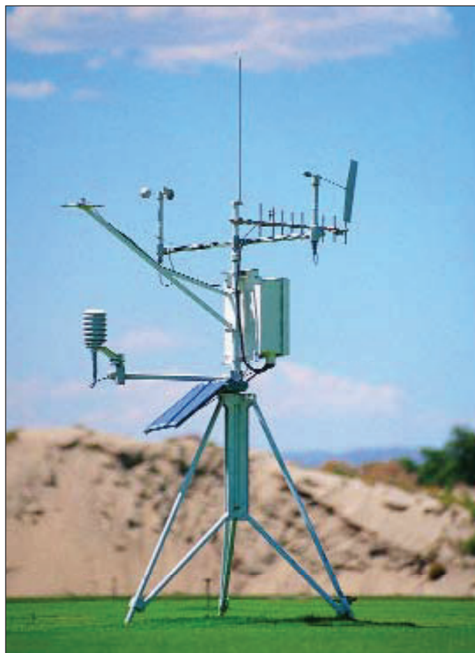
A CIMIS station gathers local weather information and sends it to Sacramento for analysis. This information is then distributed to local irrigators.
