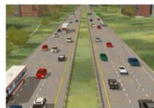
LOS B: Reasonably free flow, but speeds beginning to be restricted by traffic conditions.
